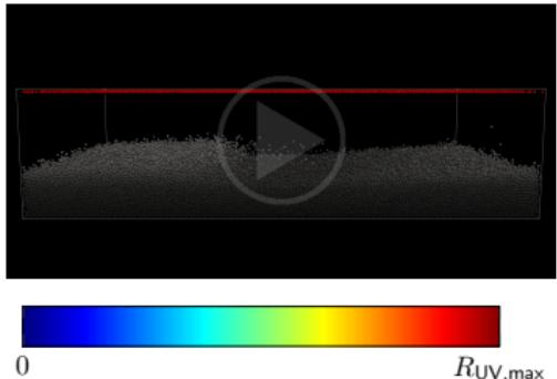
$$\begin{array}{ll} Re_b = 3000, & \text{dunes, layer,} \\ Ga_c = 20, & Ga_s = 28, \\ \rho_c^* = 1.75, & \rho_s^* = 2.5, \\ N_{p,c} = 2000, & N_{p,s} = 127070 \\ N_{\text{proc}} = 288 & t_{\text{cpu}} \approx 250000 \text{h} \end{array}$$
